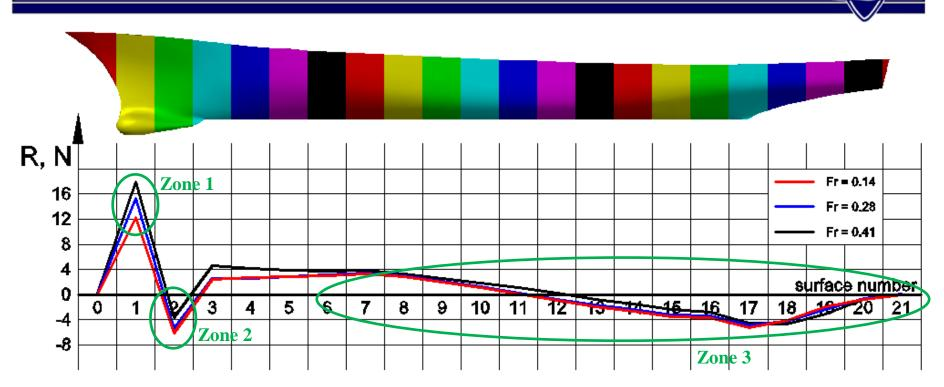
Zone 1: Maximum peak of resistance force on the nose part of the bulb; Zone 2: Minimum peak of resistance force on the stern part of the bulb; Zone 3: Approximately the same value of resistance force.
