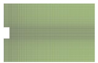
Part of mesh, 40 cells per diameter (built with SALOME)
